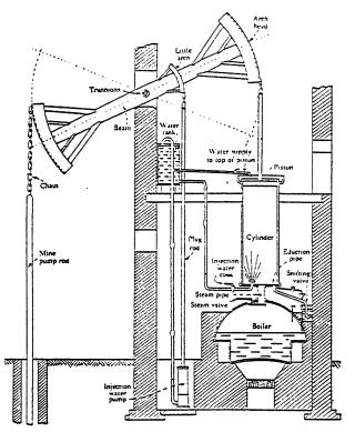
FIGURE 104—Diagram of Newcomen's atmospheric engine, 1712.
