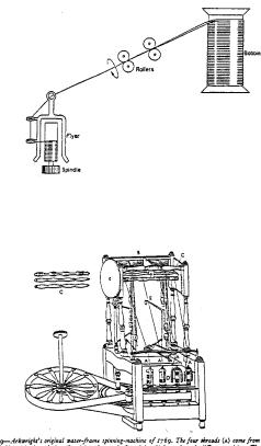
FIGURE 149-Arkwright's original water-frame spinning-machine of 1769. The four threads (A) come from the rowing boldsins (B), through the rollers (C) and on to the flort (D), which are those in different positions. The pairs of rollers (shown enlarged at the side) are pressed together by the weights (S).
