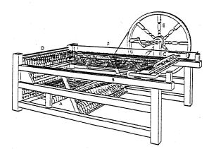
FIGURE 150—Hargreaves's spinning-jenny after it had been improved by Haley, who made the roller (A) of sheet tin for the take of lightness, and placed the wheei (E) in a vertical position. The thread passes from the rowing bobbins (B) through the clasp (C) to the spindles (D). These are rotated by bands from the roller (A), which is turned by the large wheel (E). The failer cord (F), when pulled, presses down the transverse wire (below D).
